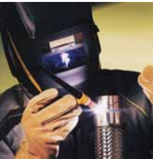
Suitable for 300 and 400 series welding. Used for stainless steel welding rods (MIG, TIG).
